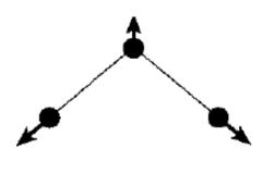
Symmetric stretch  $v_1$   $3650 \text{ cm}^{-1}$
